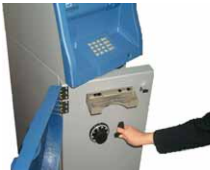
Fig.5.1a Opening the Security Door
